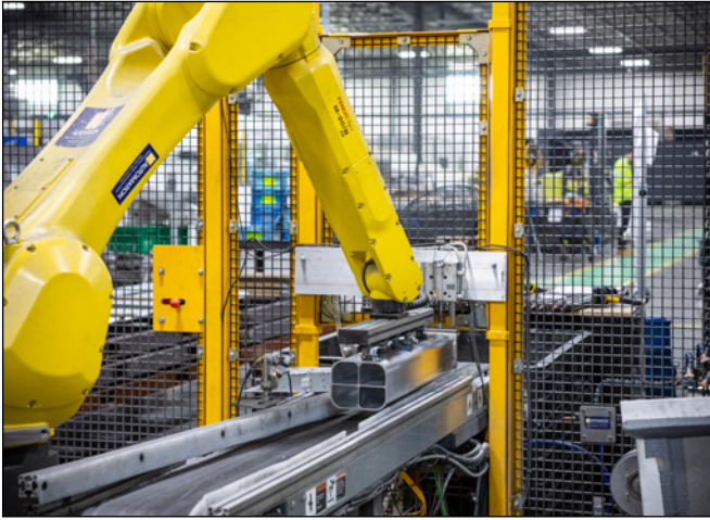
Figure 2. Automated robotic work cell for the fabrication of extruded profiles.
