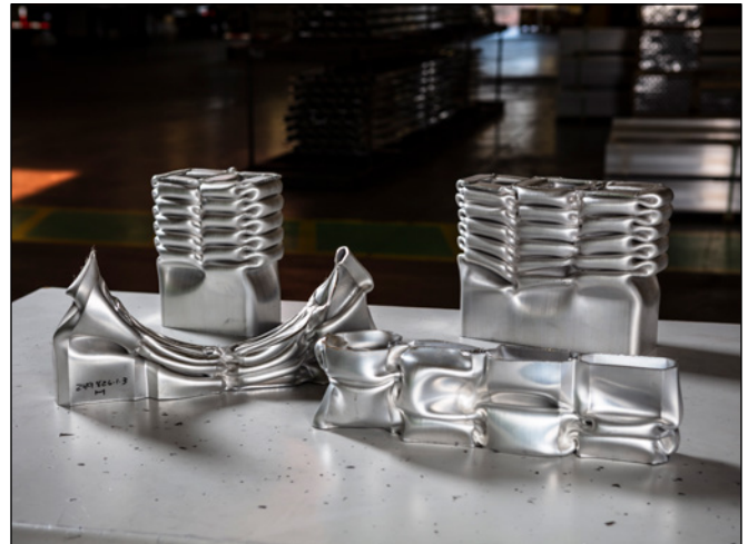
Figure 1. Crush testing of custom alloy extrusions for crash management systems.
