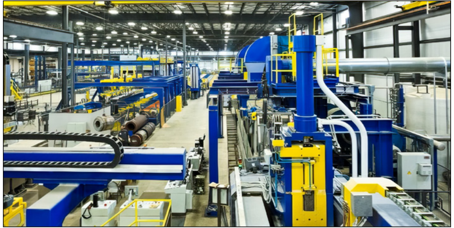
Figure 1. A new 6,500, 12 inch automotive extrusion press line was installed at Pennex in 2016.
