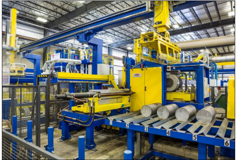
Figure 1. The billet pre-heating line for a 6,500-ton, 12 inch automotive aluminum press at Pennex.
