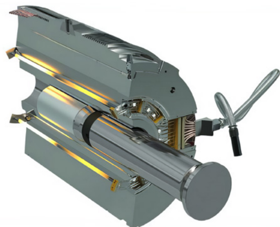
Figure 2. Example of a container with thermal intelligent controls. (Source: Castool.)
