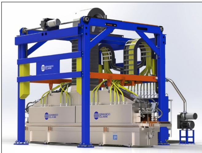
Figure 3. Example of a high pressure quenching system. (Source: Granco Clark.)
